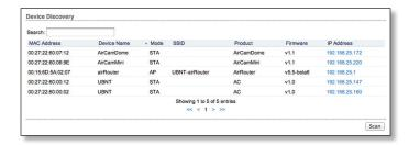
It reports the MAC Address, Device Name, Mode, SSID, Product type, Firmware version, and IP Address for each Ubiquiti device. To access a device configuration through its web management interface, click the device's IP address.
